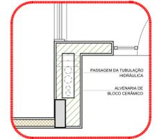
**5 DETALHE - SHAFT HIDRÁULICA**
